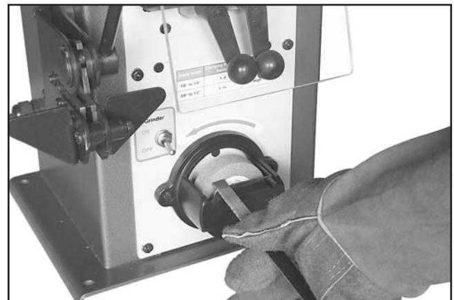
Figure 10. Using the grinder.
